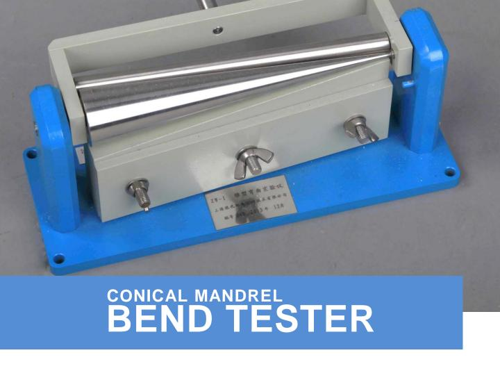
Conical Mandrel Bend Tester is applicable to evaluate crack resistance and detachment from the metal substrate of coated surface which are clamped in position and formed round the conical mandrel by rotation of the roller frame. Complying with ASTM D522-60 (1979), it is also applicable to evaluate resistance to cracking (flexibility) of attached coating on the substrates of sheet metal when elongated.
