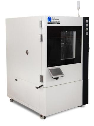
The Environmental Chamber can simulate different test environments such as temperature, relative humidity, air change and real indoor environment to determine the emission rate of formaldehyde and characteristics of various indoor materials or products.
