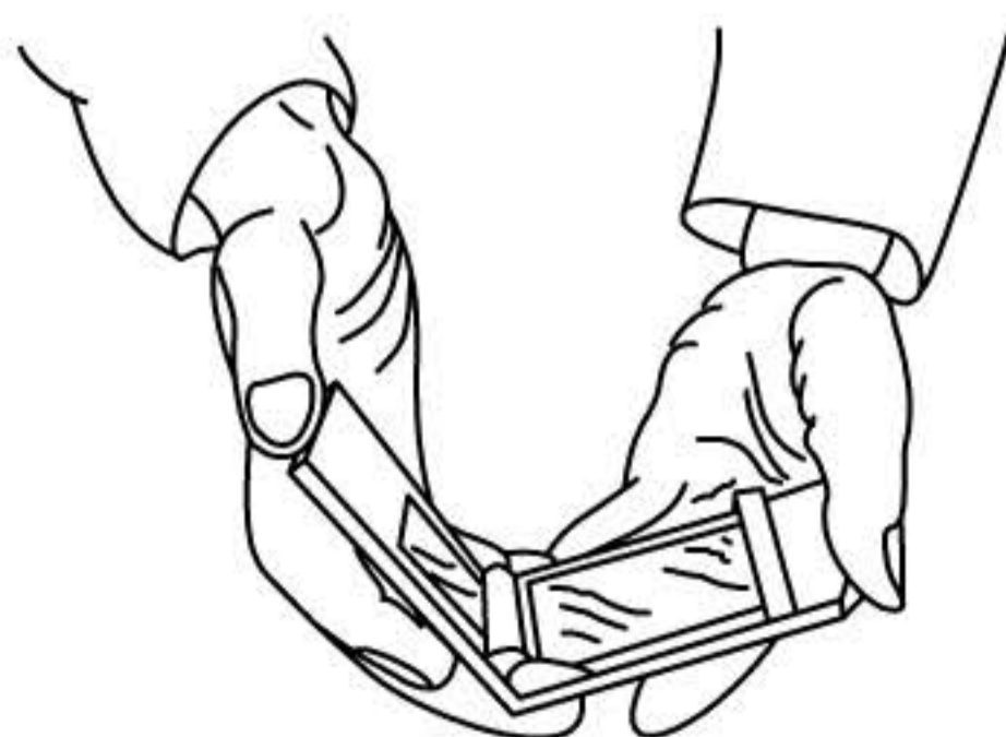
Figure 2 — Type 1 bend test apparatus in use
