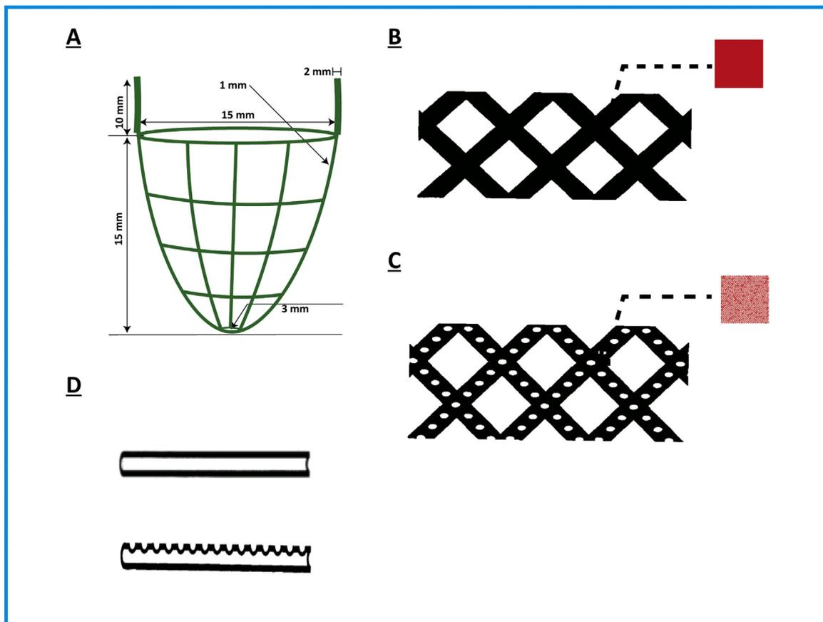
Fig. 1. Different view angles of ASD. A. dimensions of ASD, B. outer and inner lining of tubules, C. inner lining of tubules, D. cross section area of tubules.
