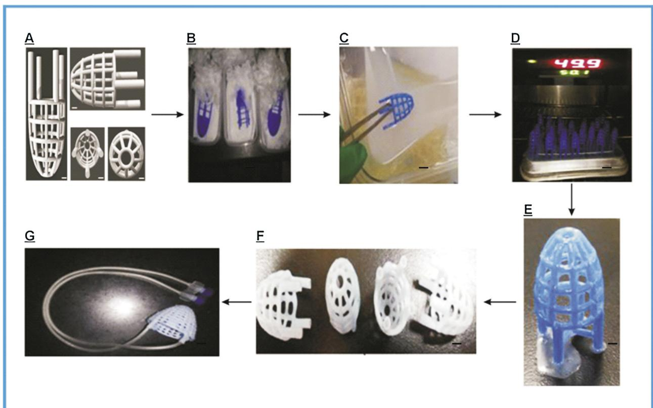
**Fig. 2.** ASD fabrication **A.** 3-D model of ASD, **B.** 3-D blue wax model, **C.** Wax model of ASD was plunge into liquid silicon, **D.** Model put into oven for 1 h at 50 °C, **E.** Blue wax start melting from the ASD model at 100 °C for 30 min, **F.** ASD from pure silicon, **G.** ASD connected with implantable catheter, scale bar 100 μm.
